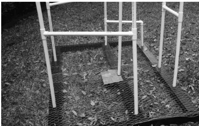
Figure 10 — PVC framework prior to installation of the TASH antenna element.
