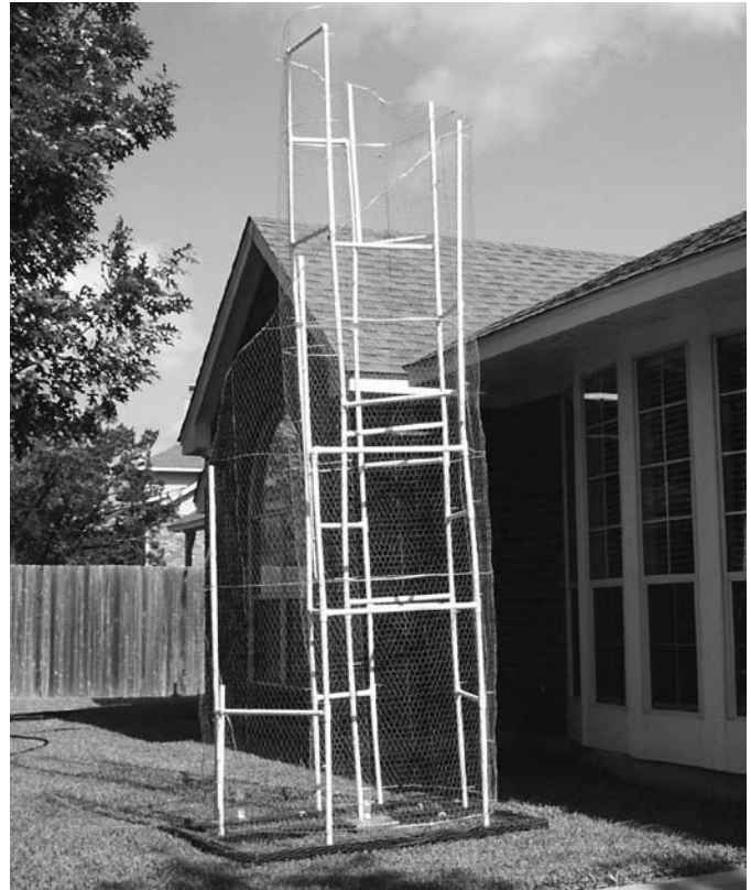
Figure 14 — Complete HF through VHF TASH antenna ready for operation.
